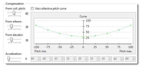
In the *Compensation* frame you can adjust factors to support the governor and compensate the different loads of the drive caused by collective and cyclic control commands in advance.
