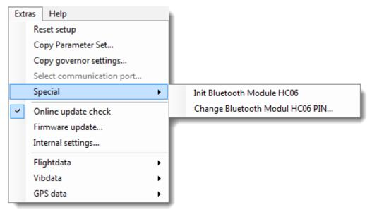
The submenu *Special* contains items, which are of interest associated with the special port. See also section **Bluetooth module** and **GPS module**.
