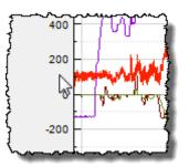
If you click with the left mouse button on the Y-axis label and hold the button, you can change the scaling of the Y axis by moving the mouse up and down.
