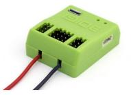
The 3Digi HC variant (HC = high current) has 2 additional cable for direct connection of the external power. These cables have a sufficiently large cross section so that there is almost no loss of voltage between BEC and 3Digi even with power-hungry servos. The cables can be fitted out with various plugs or sockets. We recommend, for example, 2mm or 3,5mm gold contact plugs.
