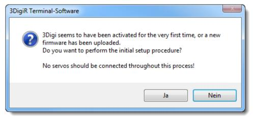
If the 3Digi is taken in operation for the first time and connected to the setup software, the above message may appear, which should be confirmed with **Yes**.
