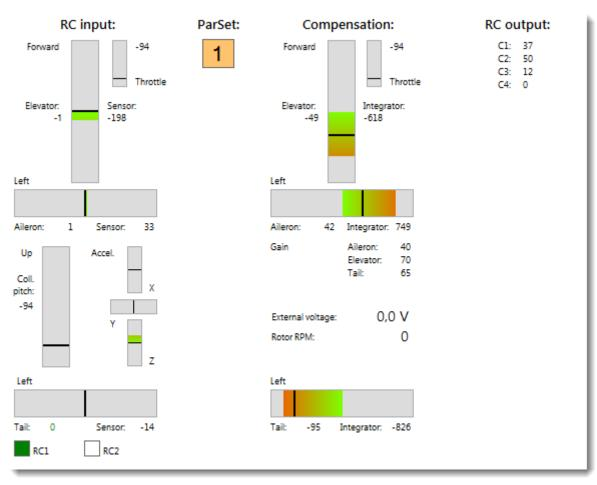
On the left side the inputs (transmitter, gyro and acceleration sensors) are displayed. In the middle you can see the outputs and the values of the integrators (I-part).
