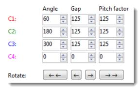
With these input fields you can individually for every servo (C1 to C4) set an **Angle**, the **Gap** between the pivot point and the rotor shaft and the collective **Pitch factor**, which the servo channel should put out.
