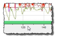
If you click with the left mouse button on the X-axis label and hold the button, you can move the mouse left and right to change the scaling of the X axis and zoom in or out certain areas.
