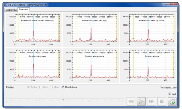
The Vibdata analysis also has an overview, in which the data of all sensors can be displayed simultaneously. The precondition is that a recording of all sensors has been made.
