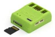
On the back is the slot for the SD card. This should be inserted into the slot with the contacts on the card facing upwards. Then push it in until it stops. The card snaps in then. The card is removed by again pressing it in and will then get unlocked. The card can then be removed by simply pulling it out.
