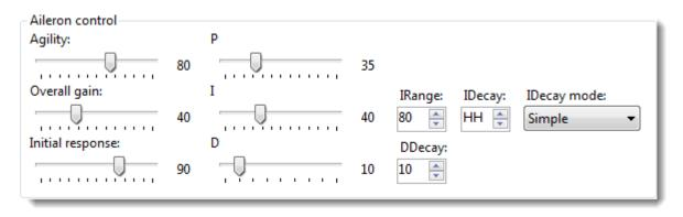
**Agility**: Specifies how fast the helicopter rotates about the specified axis, i.e. how agile he is. The rotation rate is set by the respective aileron or elevator channel on the transmitter, therefore the maximum value also depends on the servo travel/dual rate set there for the channel.
