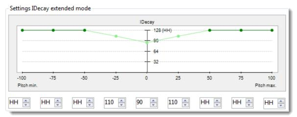
If the value "Extended" is selected in the combo box *IDecayMode*, the values here will be enabled and you can make changes here.
