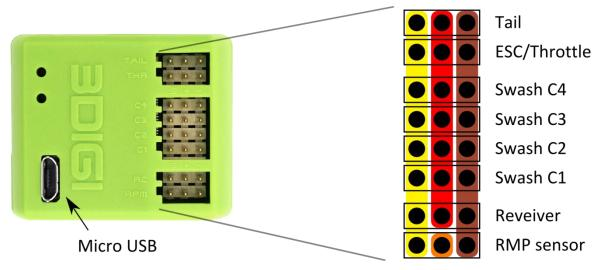
On the right side of the picture above, the inputs and outputs, that are located on the upper side of the 3DigiR, are shown schematically.
