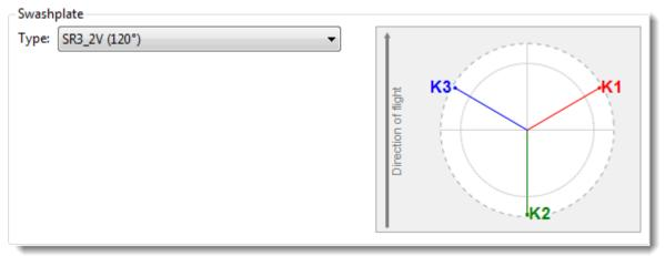
With the input fields in the frame *Swashplate* you can define the arrangement of the servos for the control of the swashplate.
